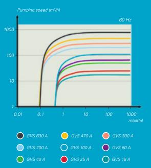
\* With gas ballast closed. Pump performance measured at the inlet pressure and 20°C. Accuracy is \*/- 10%.
